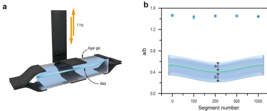
**Figure S13.** The schematic (a) and result (b) of cyclic deformation test of a Wet-MFNP in agar gel.
