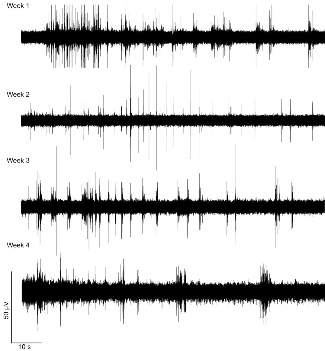
**Figure S19.** Neural signal recording of a MFNP *in vivo* for 4 weeks.
