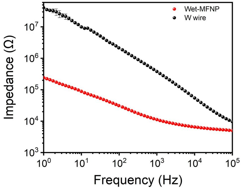
**Figure S14.** Impedance spectra of the Wet-MFNP and W wire.
