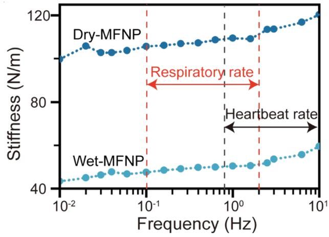
**Figure S8.** Measured bending stiffness of a Wet-MFNP and a Dry-MFNP at different frequencies with respiration and heartbeat frequencies covered in the testing range. The displacement amplitude was set as 50  $\mu\text{m}$ .
