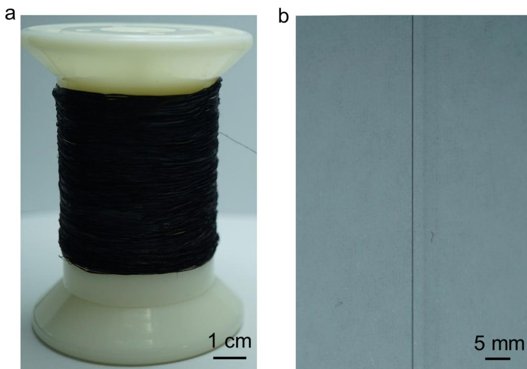
**Figure S1. a,** Photograph of a roll of the CNT fiber. **b,** A twisted CNT fiber.
