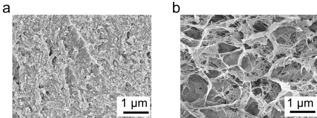
**Figure S6.** Scanning electron microscope (SEM) images of the internal structure of (a) a direct dry fiber and (b) a wet fiber by freeze drying.
