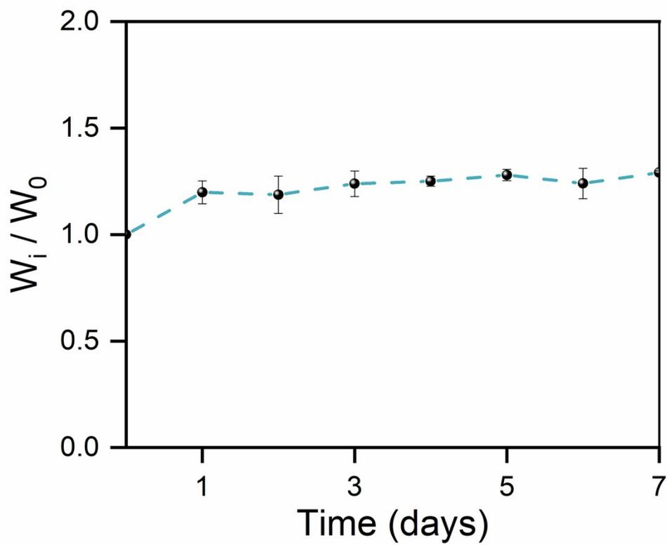
**Figure S18.** Stability of  $\text{Ca}^{2+}$ -crosslinked sodium alginate hydrogel layer *in vitro* ( $W_0$ : initial weight;  $W_i$ : weight after  $i$  days).
